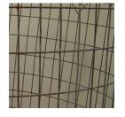
Use 2mm thick hardware wire cloth with 1" x 2:" mesh openings to allow for hatchlings to escape.
